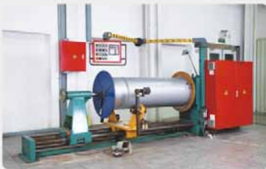
STOLLBERG高压自动绕线机 HV winding machine from Stollberg
