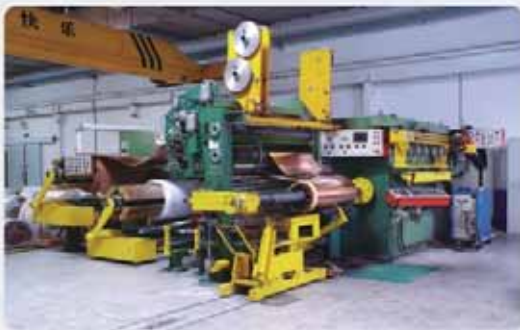
STOLLBERG低压箔式绕线机 LV foil winding from Stollberg
