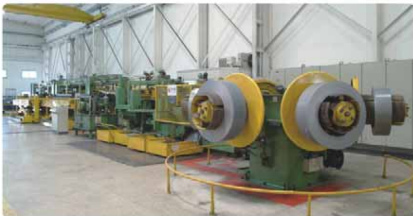
GEORG横剪线 GEORG lamination cut-to-length line
